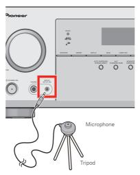
If you have a tripod, use it to place the microphone so that it's about ear level at your normal listening position. Otherwise, place the microphone at ear level using a table or a chair.
